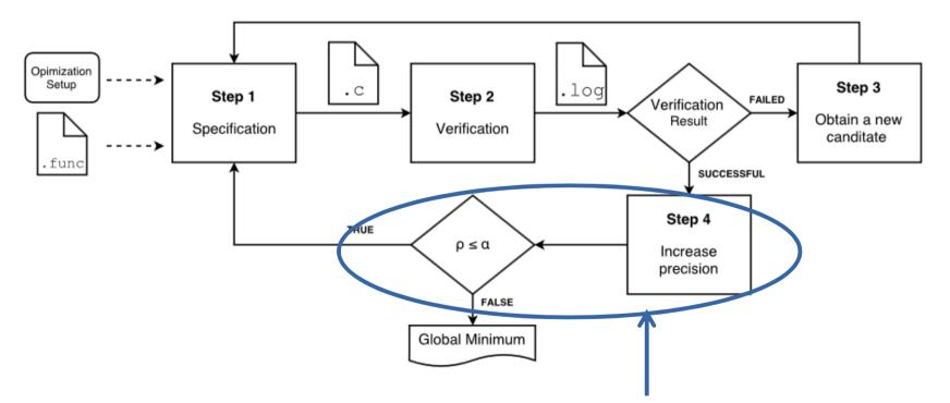
Precision is incremented and checked if it still belongs to the desired precision limit
