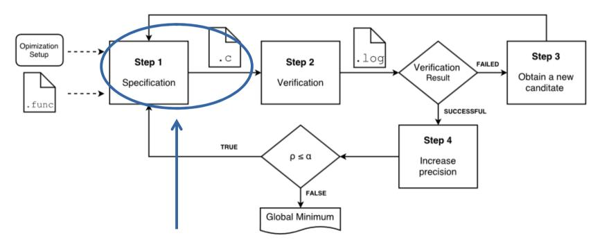
The value found is used to specify a new C file, The new candidate function value is used as the start of the algorithm
