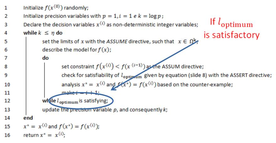
Data: A cost function f(x), a set of constraints  $\Omega$ , and a desired precision  $\eta$ . Results: The optimal decision vector  $x^*$  and the optimal cost function  $f(x^*)$ .
