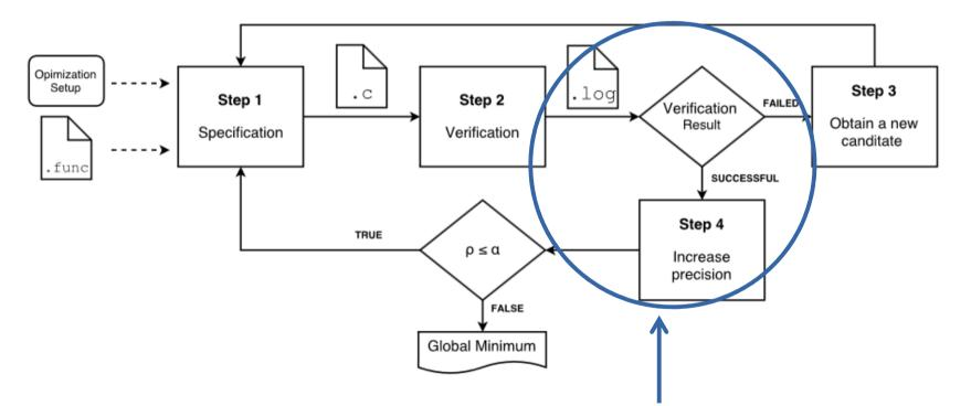
When the check is SUCCESSFUL, it means that we have found the global minimum of the function with the defined precision
