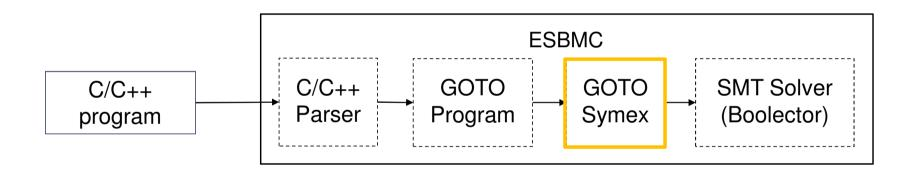
**GOTO Symex:** performs a symbolic execution of the program and generates SMT equations for constraints (*C*) and properties (*P*)
