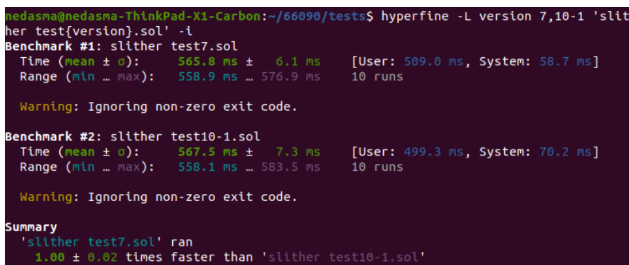
Figure 3.10: Hyperfine benchmarking tool performing tests on commands
