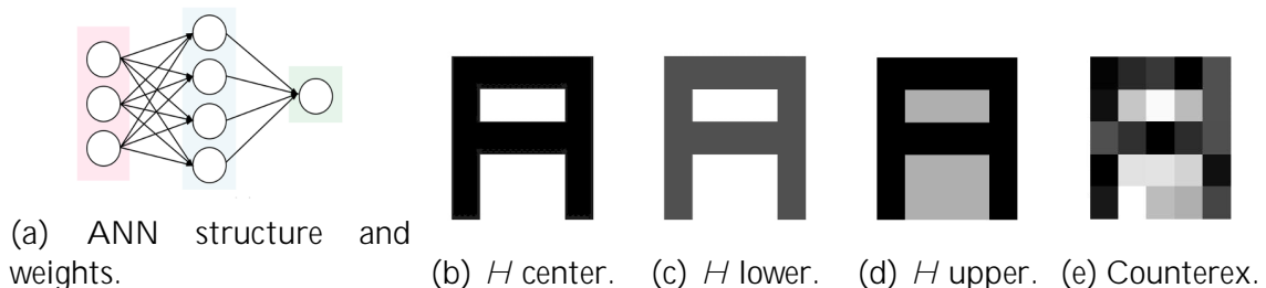
Figure 3.6: Inputs and outputs of our verification approach: (a) ANN implementation; safety property, where the (b) center, (c) lower, and (d) upper extremes of the input region are shown; and (e) a counterexample that violates the safety property.
