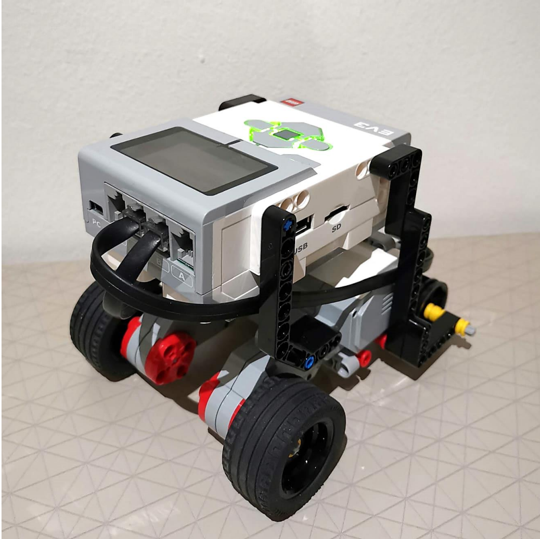
Picture 1. Robot built with Lego Mindstorms EV3 kit
