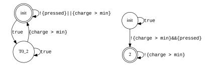
Fig. 3 The left BA accepts the example from the introduction,  $G(\{pressed\} \rightarrow F\{charge > min\})$ . The right BA is its negation, used for the *never claim* in our monitor.
